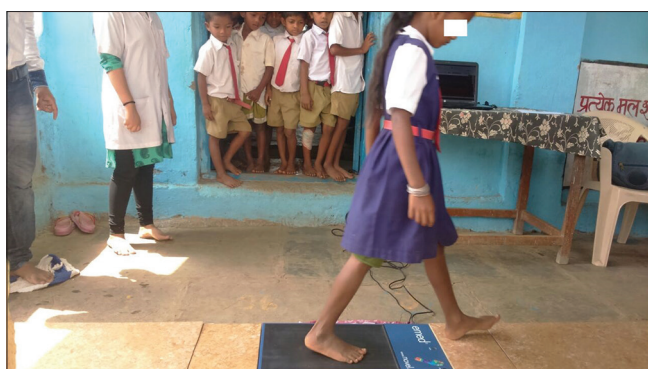
Figure 1: Use of EMED platform for measuring foot structure and pressures
