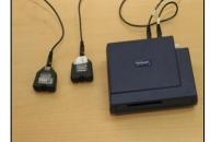
functions. It detects steps for a wide variety of normal and abnormal gait style and cadence ranging from a slow shuffle to a fast run. It has a capacity to monitor and store data for a month
