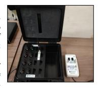
pin sensor inputs with two channels sampled at 2048 s/s and six channels sampled at 256 s/s. The ProComp Infiniti encoder is able to render a wide and comprehensive range of objective physiological signs used in clinical observation and biofeedback. All sensors are completely noninvasive and require little or no preparation for use.
