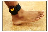
The Step Activity Monitor (SAM) by Orthocare Innovations is a highly accurate ankle worn ambulatory activity monitor, the
